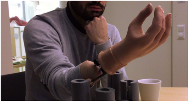
Photo above Patient with below-elbow amputation with an artificial joint that allows for natural wrist rotation.
