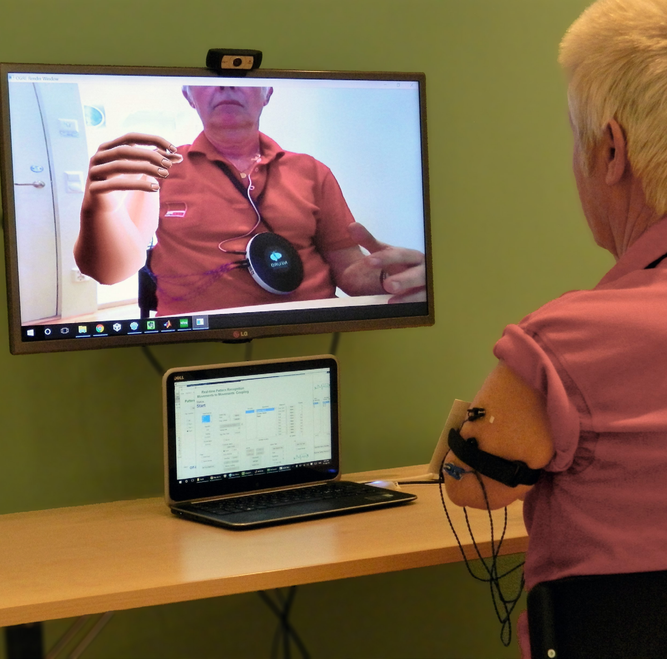
Photo right page Phantom Motor Execution (PME) as a treatment of PLP. Phantom movements are decoded using surface EMG via machine learning algorithms to be then showed in real-time using augmented reality.
